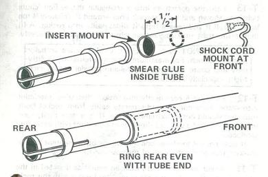
8. Glue the rear body to the main body (at the end opposite the shock cord mount). Smear glue around the inside of the main body to cover an area about 1-1/2" to 2" from the end of the tube. Immediately insert the rear body assembly, pushing it in with one smooth motion until the back of the rear ring is even with the end of the body as shown.
