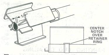
10 When the glue on the secondary fins has dried a few minutes, attach the main fin assemblies. The rear of each main fin should be even with the rear location mark, with the notch approximately centered over the retainer ring. Be careful to position the main fins to the same side of their alignment lines as the secondary fins were from theirs so all fins are spaced evenly around the body as shown in the next illustration.
