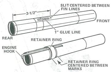
4 Cut a 1/8" long slit in the rear body at the engine hook mark as shown. Apply a 1" long line of glue to the tube running rearward from the slit. Push one end of the engine hook (p. D) into the slit and press the main part of the hook into the glue. Apply a line of glue around the tube between the two retainer ring location marks. Slide the retainer ring (part E) onto the tube, over the engine hook, and onto the glue, centering it between the two marks.
