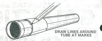
**3** Cut out the measuring guide from the pattern sheet and, using it, mark the rear body at the points indicated. Position the marks halfway between two fin lines. Use one end of the marking guide as a guide to draw a line all the way around the tube at all marks except the engine hook mark.
