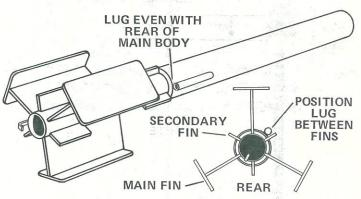
11 Glue the launch lug (part I) to the main body, centered between a main fin and a secondary fin. The rear of the lug should be even with the rear of the main body. Sight through the lug as you position it; make sure that it is straight on the body and between fins.
