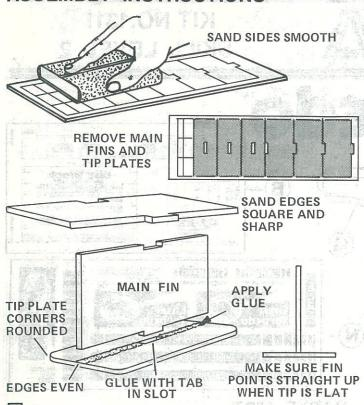
1 Sand both sides of the balsa sheet (part A) with extra fine sandpaper until smooth. Carefully remove the main fins and tip plates, using a sharp knife or single edge razor blade to free the edges. Sand the edges of the fin pieces slightly to remove any rough spots, but leave the edges square and sharp. Round the corners of the tip plates slightly. Glue a main fin to each tip plate as shown. Make sure the assemblies are square, then set them aside to dry.
