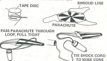
13 Cut out the parachute (part J) on its edge lines. Cut three 24" lengths of shroud line (part K). Attach line ends to the top of the parachute with tape discs (part L) as shown. Pass the shroud line loops through the screw eye on the nose cone (part M). Pass the parachute through the loop ends and draw the lines tight against the screw eye. Set the knot with a drop of glue. Tie the free end of the shock cord to the screw eye.
