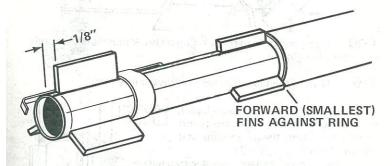
Garefully remove the secondary fins from the balsa sheet. Sand their edges square and smooth. Glue the secondary fins to the rear body, positioning them <u>next to</u> alternate (every other) alignment lines. The smaller fins are glued to the tube even with the adapter ring; the larger ones are positioned with their rear ends on the rear location mark. Smaller fins should be next to the same alignment lines as the larger secondary fins.
