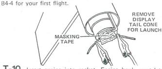
T-10 Insert engine into rocket. Engine hook must latch securely over end of engine.
