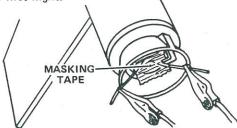
T-10 Insert engine into rocket. Engine hook must latch securely over end of engine.
