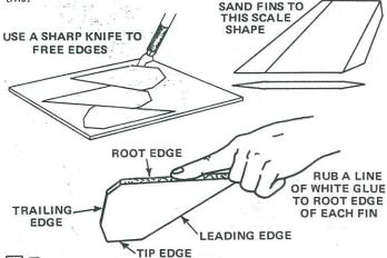
7 Fine sand the die-cut balsa sheet (part G), then carefully remove the fins from it. Free the edges with a sharp knife. For semi-scale appearance, sand the leading, trailing, and tip edges of the fins round. For full scale appearance, sand the fins as shown in the illustration. Leave the root edge of each fin square so that they can be properly glued to the body tube. Rub a line of white glue into the root edge of each fin and set aside to dry.
