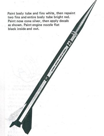
■ 18 Apply the decals (part M) to the model as shown in the photograph. To apply the water transfer decals, cut out an individual section of the decal and dip in lukewarm water for about 10 seconds. When the decal slides freely on the backing paper, slip it from the backing sheet onto the model. Use tissue paper to blot away any excess water and allow the decals to dry completely. Once the decals are dry, it is recommended that the entire model be given a light coat of clear paint to protect it.
