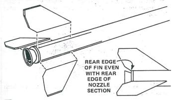
11 Glue the fins to the body tube on the fin alignment lines drawn in step 3. Refer to the illustration to be sure you position the fins correctly. Adjust the fins so they project straight away from the body tube. Do not set the rocket on its fins while the glue is wet.
