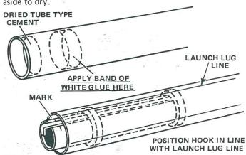
8 Test fit the engine mount assembly into the rear of the body tube. It should slide in easily. If not, sand the outside of the adapter rings until a smooth fit is achieved. Remove the engine mount and apply a band of white glue around the inside
