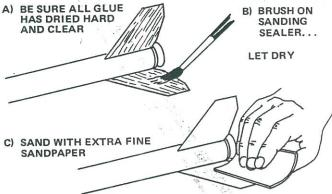
REPEAT (A&B) AS NECESSARY TO COMPLETELY FILL PORES IN WOOD
