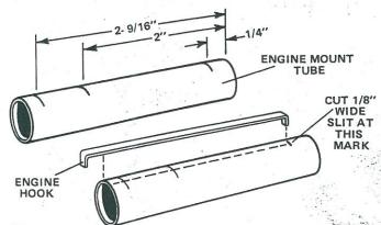
1 Mark the engine mount tube (part A) 1/4 inch, 2 inches and 2-9/16 inches from one end. Use a pencil and make the marks about 1/4 inch wide. Use a sharp knife to cut a 1/8 inch long slit at the 1/4 inch mark as shown. Push one end of the engine hook (part B) into the slit and position the hook flat against the tube.
