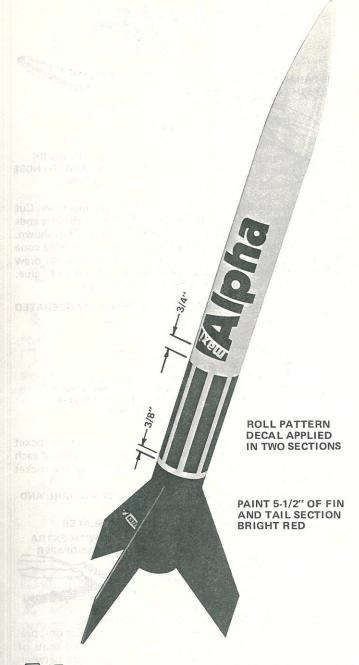
17 When all the paint is dry, apply decals (part R & S). To apply the water transfer decals, cut out an individual section of the decal and dip in lukewarm water for about 10 seconds. When the decal slides freely on the backing paper, slip it from the backing sheet onto the model.
