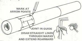
9 Cut out the tube marking guide from the pattern sheet (part K). Wrap it around the rear of the body. Mark the tube at each arrow point, front and rear. Draw a straight line connecting each matching front and rear mark. (Use a ruler when drawing lines.) Extend the launch lug line forward 14".
