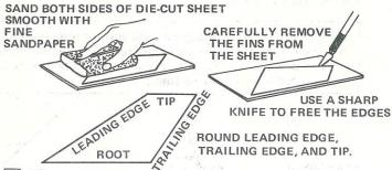
10 Fine sand the die-cut balsa sheets (part L), then carefully remove the fins from the sheets. Free the edges with a sharp knife. Sand the leading, trailing, and tip edges of the fins round. Leave the root edges square.
