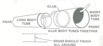
8 Smear a band of glue around the inside of one end of the forward body tube (part J), about 1/4" from the end. Slide this end of the tube over the tube coupler attached to the main
