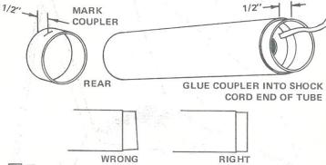
7 Mark the tube coupler (part I), 1/2" from one edge. Smear a band of glue inside the main body tube about 1/4" in from the shock cord end. Insert the tube coupler and push until the mark is even with the end of the tube. Be sure the tube coupler is installed squarely as shown.
