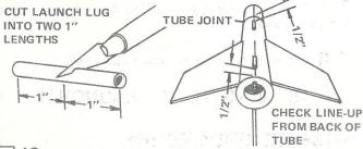
12 Cut the launch lug (part M) into two 1" lengths. Glue one of these lugs on the launch lug alignment line 1/2" from the rear of the rocket. Glue the remaining lug piece on the launch lug alignment line 1/2" rearward from the joint where the two body tubes meet. Align the launch lugs straight on the body tube.
