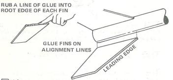
Rub a line of glue into the root edge of each fin and allow to dry. Glue the fins to the body tube on the fin alignment lines drawn in step 9. Refer to the illustration to be sure you position the fins correctly. Adjust the fins so they project straight away from the body tube. Do not set the rocket on its fins while the glue is wet.
