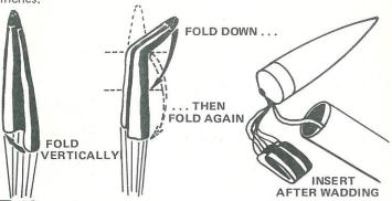
T-12 Loosely fold the parachute. Lay it on top of the wadding, with its shroud lines and shock cord on top of it. Slide the nose cone into place.
