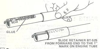
Apply a heavy line of glue on the engine hook from the 1" mark forward to the point where the engine hook enters the stuffer tube. Slip the engine hook retainer tube (part E) onto the forward end of the stuffer tube and slide it back over the engine hook to the 1" mark. Wipe away any excess glue and remove the tape from the engine hook.
