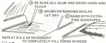
15 When all glue on the outside of the model is dry, prepare the balsa parts for painting. Apply at least two coats of sanding sealer to the fins. Let dry and sand lightly between coats. Do this until the tiny holes in the wood are filled and
