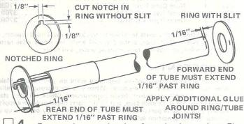
Remove the centering rings from the ring set (part F). Cut a 1/8" wide, 1/8" long notch in the ring without the slit. Place the rings on the stuffer tube as shown. The stuffer tube should project 1/16" past the centering rings at each end. Glue centering rings securely in place and allow to dry. Apply a second layer of glue to both sides of each ring for strength.
