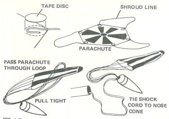
13 Cut out the parachute (part N) on its edge lines. Cut three 48" lengths of shroud line (part O). Attach the line ends to the top of the parachute with tape discs (part P) as shown. Pass the shroud line loops through the ring on the nose cone (part Q). Pass the parachute through the loop ends and draw the lines tight against the ring. Set the knot with a drop of glue. Tie the free end of the shock cord to the nose cone.
