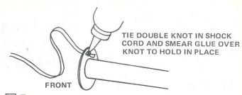
Tie a secure double knot at one end of the shock cord (part G). Slip unknotted end through the slit in the forward centering ring. Pull the knot tightly against the back of the ring as shown. Apply a heavy coating of glue over the knot to hold it in place.
