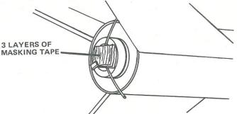
**T-11** Install an igniter in a D12-5 engine as directed in the engine instructions. Insert engine into the engine mount. Make sure the engine hook latches securely over the end of the engine.
